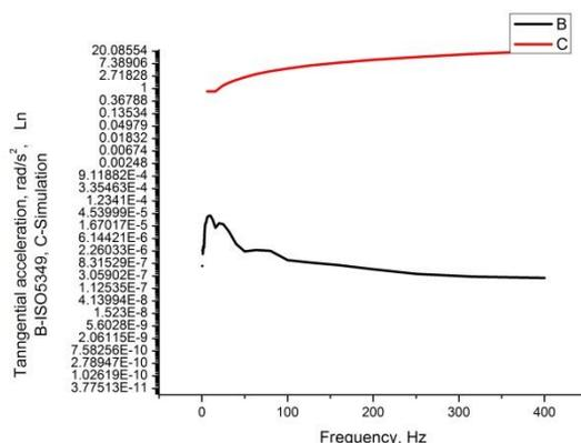
Figure 7. The comparison of ISO 5349/DIS criteria and calculated tangential accelerations (the ordinate axis is logarithmic due to small values of tangential accelerations).
