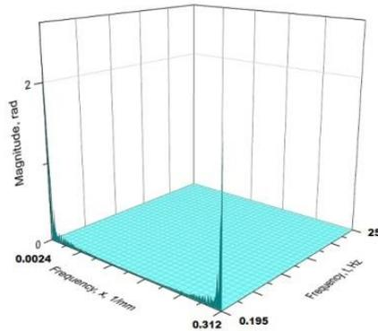
Figure 5. Spectrum magnitude of torsional vibrations of the steering shaft
