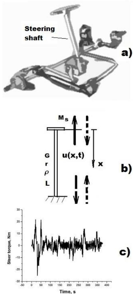
Figure 2. Observed concept of servo steering a), idealized model of the steering shaft b) and experimental torque on the steering wheel c)
