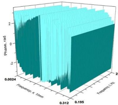
Figure 6. Phase angles of the spectrum of torsional vibrations of the steering shaft
