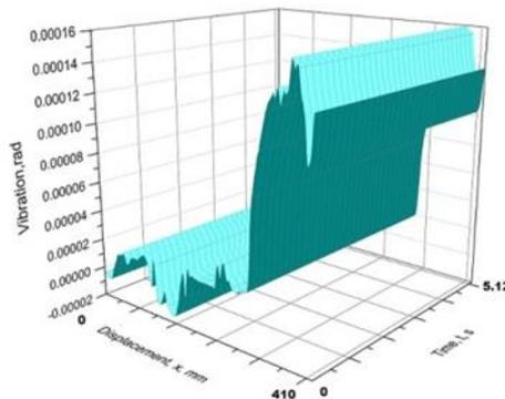
Figure 4. Torsional vibrations of the steering shaft
